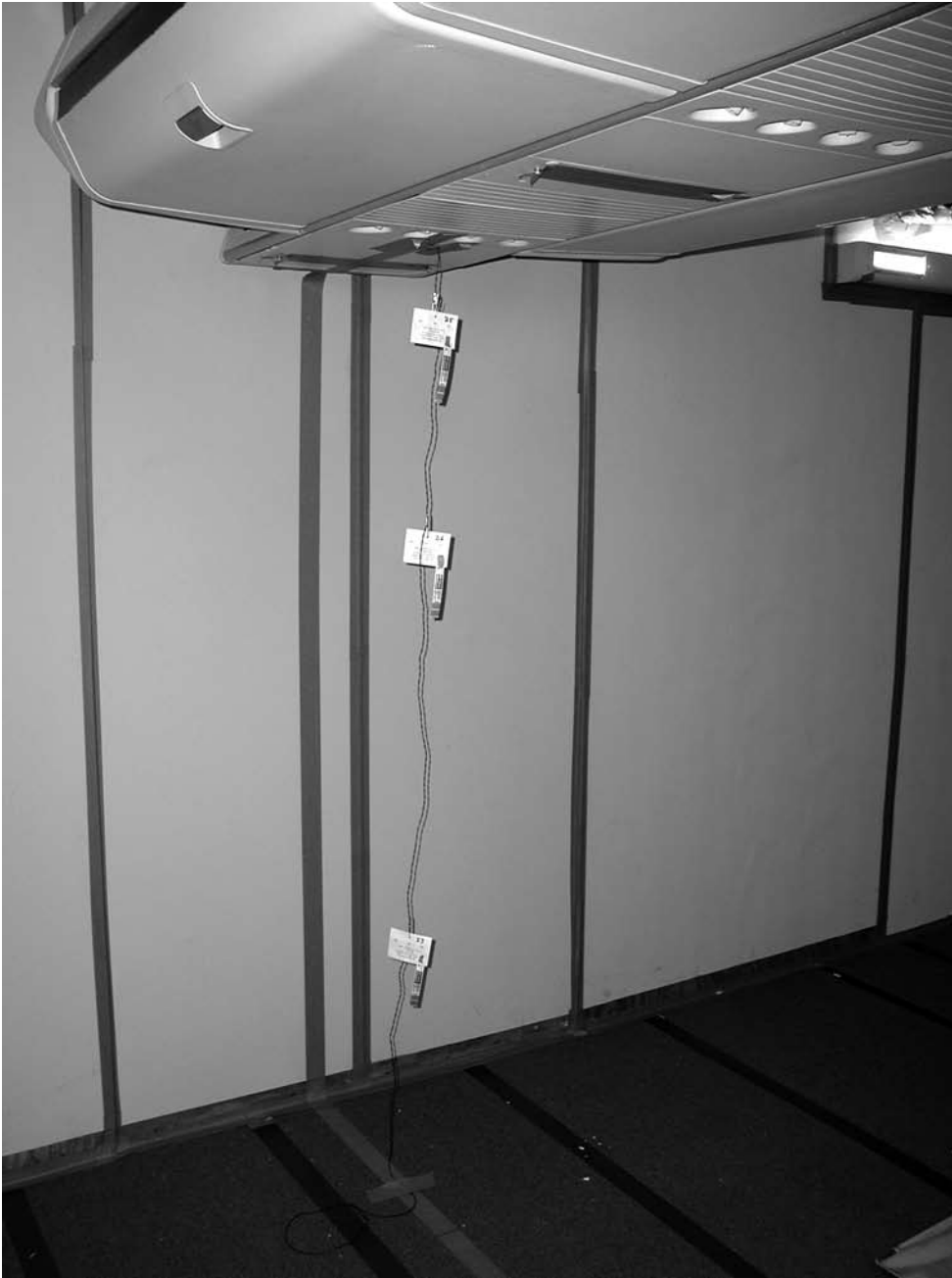
Figure 6. Photograph of BIs and CIs (positions no. 25 – 27, as shown in Figure 7 and identified in Table I) attached to wire in preparation for testing.
